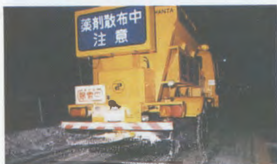
Figure 9 – Application of anti-freezing agents
